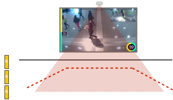
Figure 3. Wireframe of final design. Display is projected onto the wall, above which is surveillance camera. In red: field of camera vision and area within which it detects motion. Three associated kiosks line the left wall.
